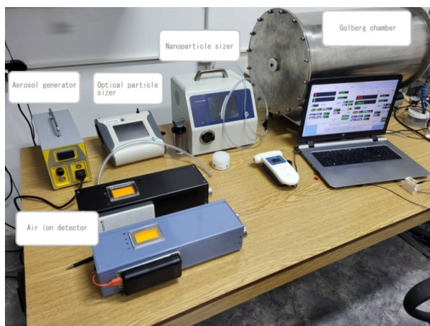
FIGURE 1. Aerosol and ion generation equipment, ozone level monitoring, aerosol particle concentration and ion concentration measurement equipment.
